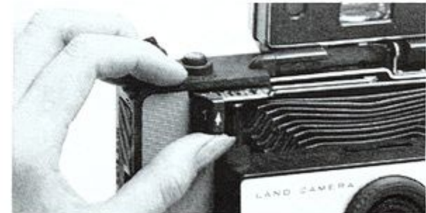
5. Raise button No. 1; this unlocks camera front.
