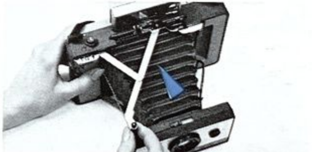
6. Pull camera front out as far as it will go.
